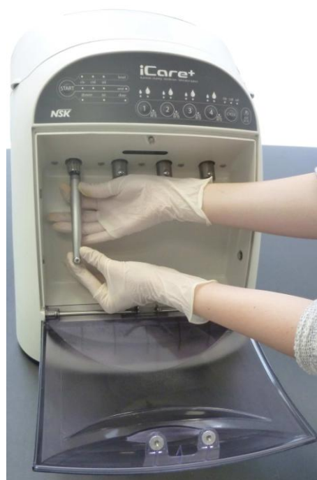
Figure 15: Screwing the ring on the Midwest coupling
