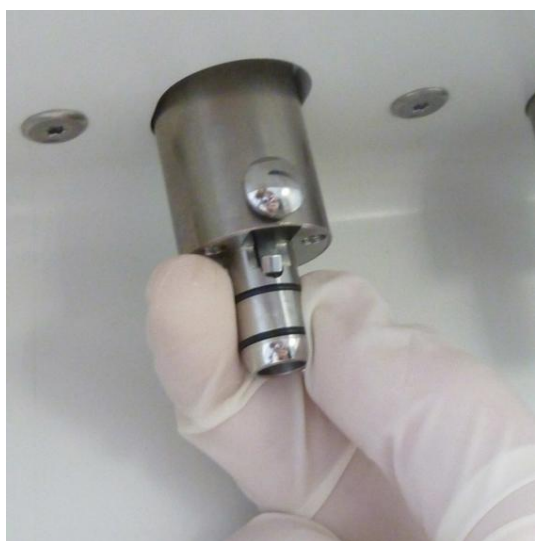
Figure 29: O-ring joints of E-type connector
