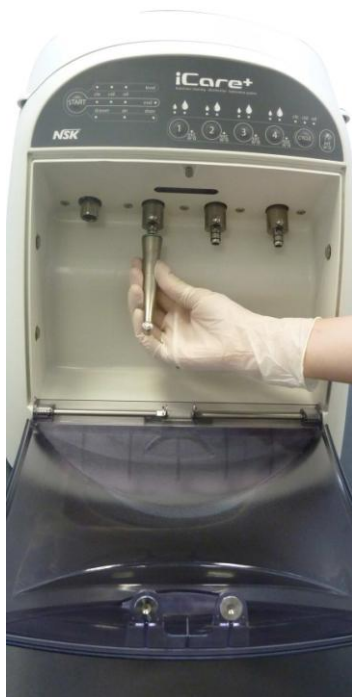
Figure 17: Connection of a contra-angle
