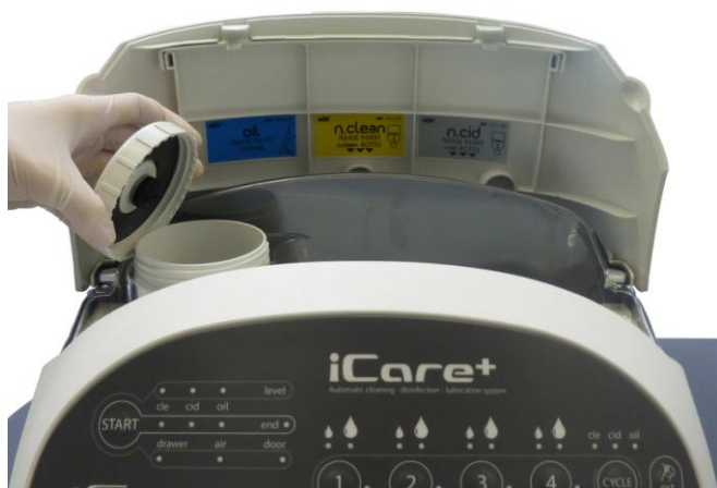
Figure 12: Unscrewing the Oil tank's cap of iCare+ device
