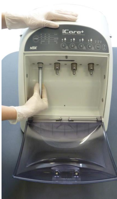
Figure 14: Connection of one turbine
