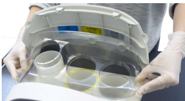
Figure 28: Replacement of the junction support blister
